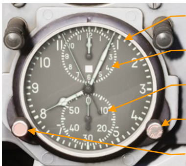
Figure 16: Air watch. AChS-1M
