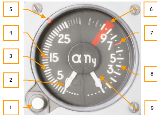
Figure 13: Combined AOA / G meter
