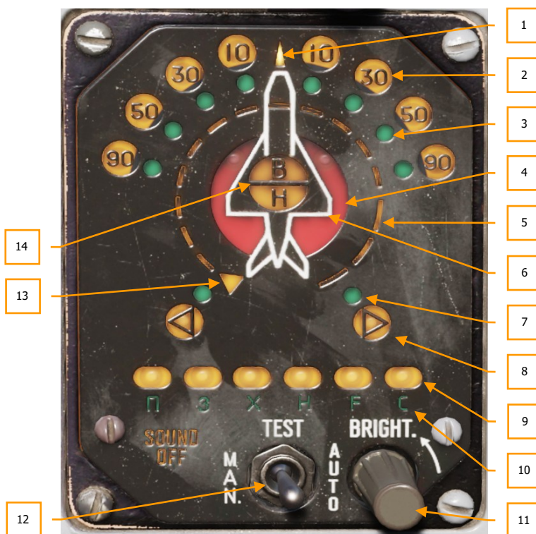
Figure 103: RHAW. SPO-15LM display unit
