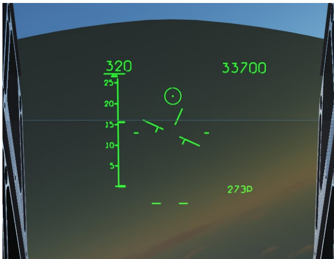
Figure 93: "OPT" mode. Manual targeting
