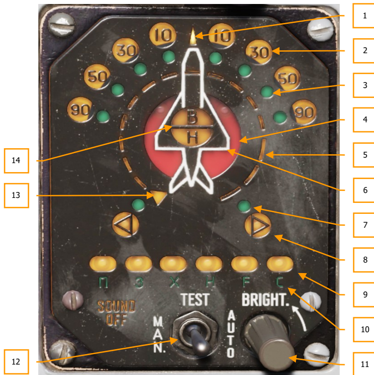
Figure 30: RHAW. SPO-15LM display unit
