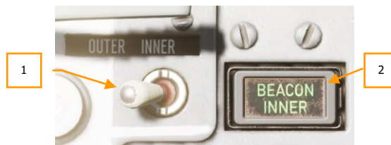
Figure 18: Toggle switch for selecting the type of NDB beacon (outer or inner)
